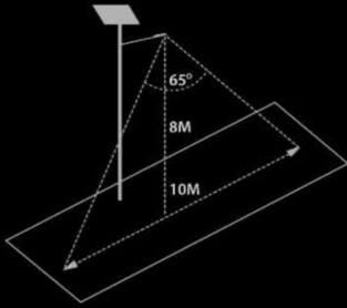
Microwave (Radar) sensor is adopted in this light in order to save more energy. Energy saving mode is adjustable by the remote control easily. Radar sensor is more senditive than PIR sensor in much wider angle and longer distance. And it can be trigered distance from people/ object to light sensor should be within 12 meters.
